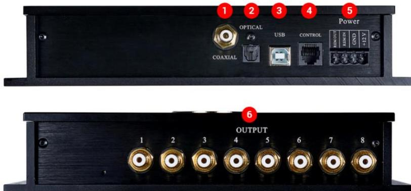
**1. Coaxial.** Electrical input for connecting SPDIF source with coaxial output. Digital thread is supported in stereo. Playback of multi-channel signal (Dolby Digital, DTS) does not support.
